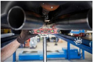
9. The tip sections can now be installed on each side. Make sure to also slide the clamp onto the muffler before doing so. Loosely position them and then snug the clamps to hold them in place as shown. The tip section alignment/orientation is primarily dictated by the positioning of mid pipe to muffler pipe sections. Ideal fitment would leave equal spacing on all sides of the tip section.
