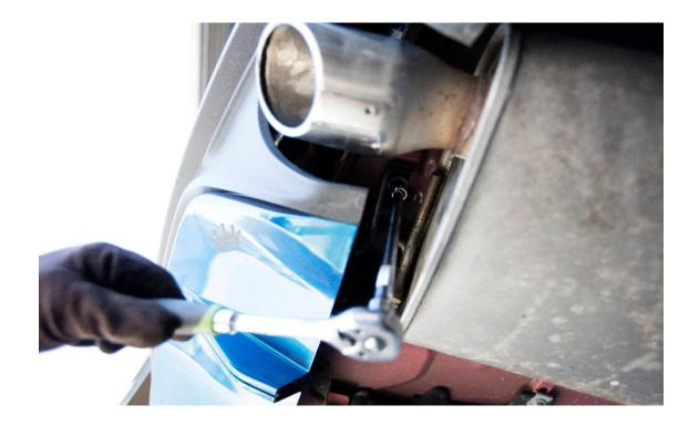
4. Next you may remove the factory rear exhaust hangers holding the system to the rear suspension just above the differential cover (x1 13mm bolt each side). These hangers can remain on the system until it is removed from the vehicle. Spray some lubricant on the rubber portions as you will need to remove these and reinstall on your new Krona system.
