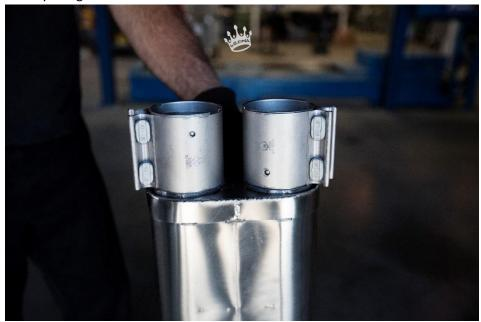
3. With help from another set of hands or with the use of a stand to support the mid-section, you are now ready to lift your Krona system into place (all that time at the gym has prepared you for this moment). Be sure the seamed portion of the resonator is facing upward as pictured (it looks better that way). Snug the clamps at this time just to hold everything in place, but do not tighten.
