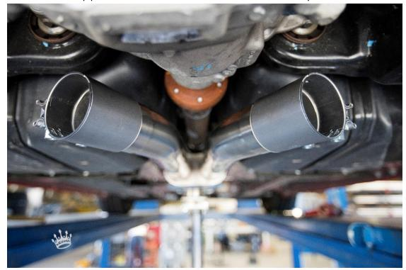
5. Now you are ready to transfer over the factory exhaust hangers. The hangers located on the differential can be loosely installed on the rear suspension. These hangers also have hooks in them to ease in putting them in their proper location.
