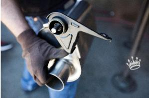
7. You are now ready to install your rear mufflers (one side at a time). Slide the muffler pipe into the clamp on the midpipes and then lift the muffler section into place. The hooks on the rear muffler hangers will ease this step of the installation. Once in place install the bolts to hold everything in place. Do not tighten just yet.
