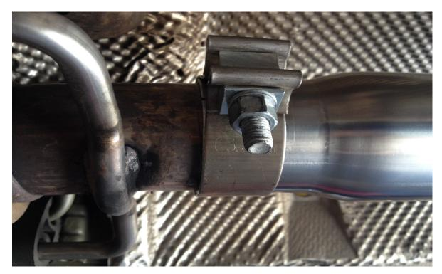
Next you may move to connecting the 3" resonator section to the Krona adapter pipe. Be sure to slip a 3" clamp over the end of the adapter pipe before making the connection.
