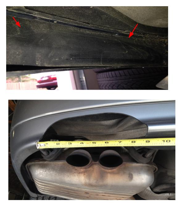
Once you have made the bumper modification you should now be getting excited... You are almost done :-)! You may now install the muffler/tip section, be sure to slip a clamp over the under axle pipe prior to making the connection. Lift the muffler into place and install the hangers in the factory location.
