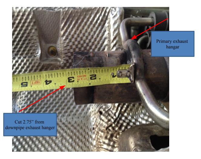
There are only 6 rubber exhaust hangers holding the OE exhaust to the vehicle (two at the OE downpipe after the flex joint, one just after the center resonator, one just before the rear muffler and two on the rear muffler. Remove the exhaust from the downpipe back by slipping the factory hangars from the rubber mounting points. With a little bit of elbow grease you can slide the factory system out from under the vehicle (If all else fails talk nice to it ;-))
