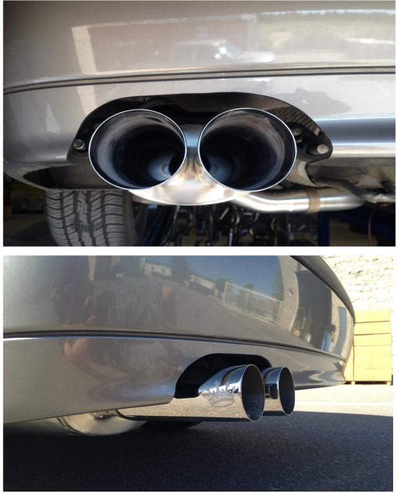
Position the muffler so that it is center perfectly in the bumper cut out. Once you are happy with its location you may now tighten all exhaust clamps starting with the muffler and working your way forward. **Torque all slip fit connections to 20 ft lbs.**
