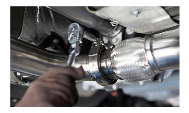
6. Ensure that all pieces are aligned and fitment is correct. Now tighten down the V band clamp and then your factory slip connection.
