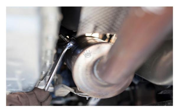
4. Next you may remove factory downpipe bracket holding it to the side of the transmission. (x2 13mm bolts) This is also an excellent time to remove the bracket from the factory downpipe (x2 13mm nuts).
