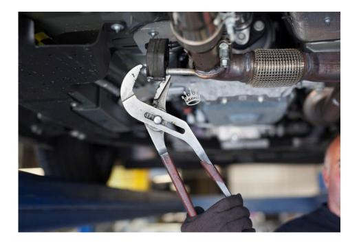
3. The secondary O2 sensor may now be unplugged and removed from under the car (7/8 wrench). This is best to unplug from the top of the vehicle.
