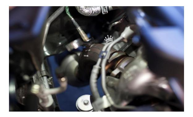
6. Your downpipe is almost ready to be removed. From the top of the vehicle you may now remove the two top turbo flange nuts using a 15mm deep wall socket or a 15mm wrench.
