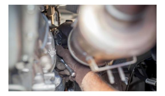
8. Everything is now loose and your factory downpipe is ready to be removed from the underside of the vehicle. Carefully slide the downpipe out of the connection with the mid pipe (this was loosed in step 2) by pulling the downpipe. It should be relatively easy to slide free.
